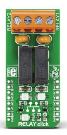
**RELAY click** can control various devices with up to 5A, 250V AC/30V DC loads. It features two <u>G6D1AASI-5DC</u> power PCB relay modules. The click is designed to run on 5V power supply only. RELAY click communicates with the target microcontroller via mikroBUS™ PWM (RL1) and CS (RL2) pins.
