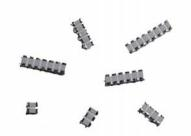
PRA arrays can be used in most applications requiring a matched pair (or set) of resistor elements. The networks provide 1ppm/°C T.C.R. tracking, a ratio tolerance as tight as 0.01% and outstanding stability. They are available in 1 mm, 1.35mm and 1.82mm pitch.
