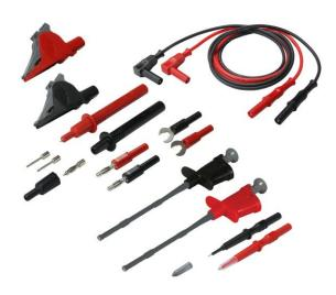
Full offering of accessories for Electrical or Electronic Applications. Both large and micro-sized probe bodies, flexible pincer clip for long reach applications, fully insulated alligator clips for over-sized lugs or fine wires, and spade lug or banana plug adapters for fixed terminal connections. All this utility while meeting the latest international safety standards.
