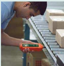
Accessory wheels enable tachometer to measure linear surface speeds
