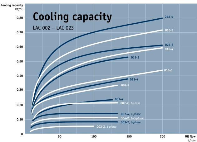
Cooling capacity tolerance  $\pm$  10% kW.
