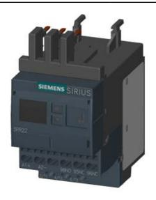
MONITORING RELAY ATTACHABLE TO CONTACTOR 3RT2. SIZE S00 STANDARD, DIGITAL ADJUSTABLE APPARENT/ACTIVE CURRENT MONIT. 1.6 - 16A, 20-400 HZ, 3-PHASE SUPPLY 24-240 V AC/DC 1 CO CONTACT, 1 SEMICOND. FOR ALARM AND WARNING MONITORING FOR CURRENT OVERSHOOT/UNDERSHOOT PHASE FAILURE, WIRE BREAK PHASE SEQUENCE FAULT CURRENT BLOCKING CURRENT WARNING AND ALARM THRESHOLDS WITH OR W/O ERROR LOG ONDELAY 0-99 S SPURIOUS PEAK SUPPR.0-30 S BREAK AFTER FAULT 0-300 MIN SPRING-LOADED CONNECTION
