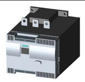
SIRIUS SOFT STARTER, VALUES WITH 575 V, 50 DEG., STANDARD: 280A, 250HP, INSIDE-DELTA CIRCUIT 3: 485A, 500HP, 400-690 V AC, 115 V AC, CAGE CLAMP TERMINALS
