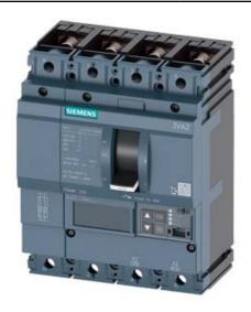
CIRCUIT BREAKER 3VA2 IEC FRAME 250 BREAKING CAPACITY CLASS H ICU=85KA @ 415 V 4POLE, LINE PROTECTION ETU560, LSIG, IN=250A OVERLOAD PROTECTION IR=100A ...250A SHORT CIRCUIT PROTECTION ISD=0,6..10X IN, II=1,5..10X IN NEUTRAL PROTECTION ADJUSTABLE (OFF, UPTO 100%) GROUNDFAULT, SWITCHABLE IG=0,2... 1 X IN, TG=0,050,8MS BUSBAR CONNECTION
