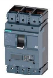
CIRCUIT BREAKER 3VA2 IEC FRAME 630 BREAKING CAPACITY CLASS C ICU=110KA @ 415 V 3-POLE, LINE PROTECTION ETU560, LSIG, IN=400A OVERLOAD PROTECTION IR=160A ...400A SHORT CIRCUIT PROTECTION ISD=0,6..10X IN, II=1,5..15X IN NEUTRAL PROTECTION OPTIONAL WITH EXT. CT;UPTO 160% GROUND-FAULT, SWITCHABLE IG=0,2... 1 X IN, TG=0,05-0,8MS BUSBAR CONNECTION
