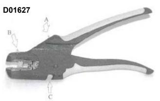
The D01627 has been designed to remove insulation from wire and cables, ideal for installation electricians. The design of the tool enables the user to strip cable of 6 mm<sup>2</sup> (10 AWG) down to 0.082 (27 AWG) with an easy action gripping pad adjuster (A) and blade depth adjuster (B) providing in the one tool what was previously only available by having several. The tool also has a cut off blade (C) handling cable up to 6 mm<sup>2</sup> (10 AWG) stranded copper conductor
