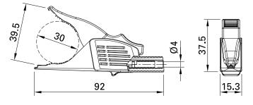
Made of brass with all-round insulation. Toothed jaws for wide grip with surface for fine wire.  $\emptyset$  4 mm rigid socket in insulator accepting spring-loaded  $\emptyset$  4 mm plugs with rigid insulating sleeve.
