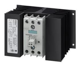
SEMI-CONDUCTOR CONTAC.3-PH.3RF2 AC51 40A 40 DEG. C 48-600V / 4-30V DC 3-PHASE CONTROLLED SCREW TERMINAL BLOCKING VOLTAGE 1200V
