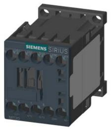
CONTACTOR, AC-3, 5.5KW/400V, 1NC, DC 48V, 3-POLE, SZ S00 SCREW TERMINAL
