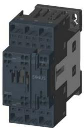
CONTACTOR, AC-3, 18.5KW/400V, 1NO+1NC, AC 24V 50HZ, 3-POLE, SZ S0 SPRING-LOADED TERMINAL
