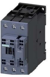
CONTACTOR,AC3:22KW/400V, 1NO+1NC, 175-280V AC/DC, WITH VARISTOR, 3-POLE, SIZE S2, SPRING-TYPE TERMINAL
