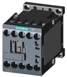
2NO+2NC CONTACTOR, AC3: 4KW AC 42V 50HZ 4-POLE, 2NO+2NC, SZ: S00, SCREW TERMINAL
