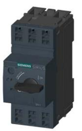
CIRCUIT-BREAKER SZ S00, FOR MOTOR PROTECTION, CLASS 10, A-REL. 0.14...0.2A, N-RELEASE2.6A, SPRING-L. CONNECTION STANDARD SW. CAPACITY
