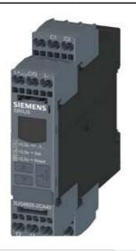
DIGITAL MONITORING RELAY FOR FAULT CURRENT MONITORING (W. DIFFERENTIAL CT 3UL23) FOR IO-LINK SETTING RANGE 0.03A TO 40A SEPARATE FOR ALARM THRESHOLD AND SWITCH-OFF VALUE STARTUP AND TRIPPING DELAY 0 TO 999.9S SWITCH-OFF HYSTERESIS UP TO 50% ALARM HYSTERESIS 5% FIXED WIDTH 22.5 MM, 2 CO CONTACTS W. OR W/O ERROR LOG SPRING-LOADED TERMINAL
