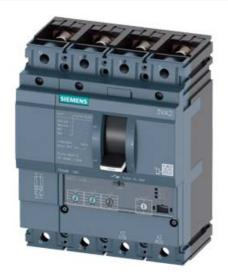
CIRCUIT BREAKER 3VA2 IEC FRAME 160 BREAKING CAPACITY CLASS M ICU=55KA @ 415 V 4POLE, LINE PROTECTION ETU320, LI, IN=25A OVERLOAD PROTECTION IR=10A ...25A SHORT CIRCUIT PROTECTION II=12 X IN NEUTRAL PROTECTION ADJUSTABLE(OFF,100%) BUSBAR CONNECTION
