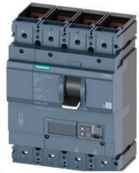
CIRCUIT BREAKER 3VA2 IEC FRAME 630 BREAKING CAPACITY CLASS M ICU=55KA @ 415 V 4-POLE, LINE PROTECTION ETU550, LSI, IN=400A OVERLOAD PROTECTION IR=160A ...400A SHORT CIRCUIT PROTECTION ISD=0,6..10X IN, II=1,5..15X IN NEUTRAL PROTECTION ADJUSTABLE (OFF, UPTO 160%) BUSBAR CONNECTION
