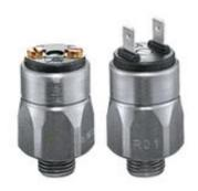
Function: The pressure switch monitors a set pressure value. It opens or closes an electric circuit when a certain (adjustable) pressure is reached.
