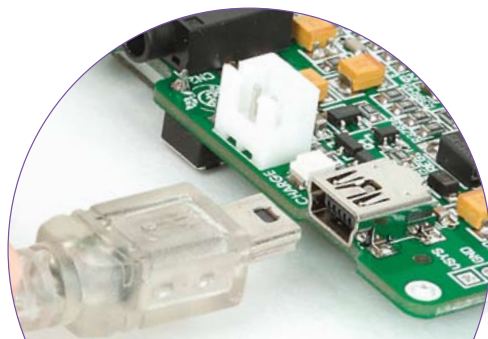
Figure 9-1: Connecting USB cable to MINI-B USB connector
