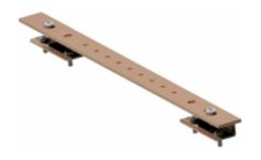
The GRDBAR Series comes in vertical, horizontal mounting as well as horizontal rack mounting. The grounding bar is made from heavy-gauge copper that attaches to the inside of an enclosure, cabinet or open frame rack to provide consolidated equipment grounds. Ground points have been drilled and tapped to accommodate a #10-32 screw (included). Use with our **Ground Wire Kits** to bond your equipment to the busbar.
