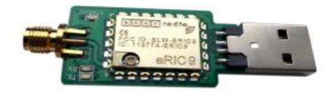
The eRIC9-USB dongle is fully USB compatible, offering customers a simple, ready-to-use and flexible modem for enabling any USB host device with 868/915MHz ISM radio communications.
