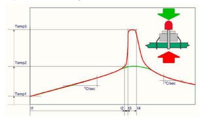
Green curve: Temperature on the component side of the pcb
