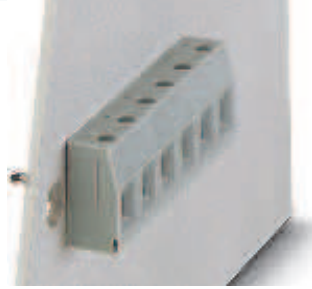
4/6 mm 2 molded feed-through terminal block, horizontal conductor connection, inside with solder connection and knurled nut
