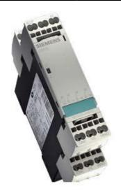
COUPLING RELAY IM INDUSTRY-STANDARD ENCLOSURE 3 CHANGEOVER CONTACTS COMBIVOLTAGE 24 V AND 220 V TO 240 V AC/DC CAGE CLAMP CONNECTIONS
