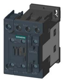
4NO CONTACTOR, AC1: 40A AC 110V 50HZ 4-POLE, 4NO, SZ: S0, SCREW TERMINAL 1NO+1NC INTEGR.
