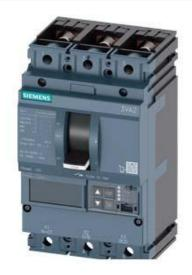
CIRCUIT BREAKER 3VA2 IEC FRAME 100 BREAKING CAPACITY CLASS L ICU=150KA @ 415 V 3POLE, LINE PROTECTION ETU560, LSIG, IN=40A OVERLOAD PROTECTION IR=16A ...40A SHORT CIRCUIT PROTECTION ISD=0,6..10X IN, II=1,5..12X IN NEUTRAL PROTECTION OPTIONAL WITH EXT. CT,UPTO 160% GROUNDFAULT, SWITCHABLE IG=0,2... 1 X IN, TG=0,050,8MS BUSBAR CONNECTION
