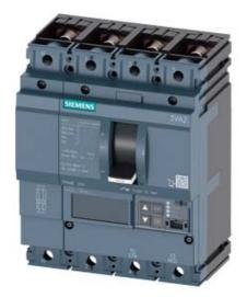
CIRCUIT BREAKER 3VA2 IEC FRAME 250 BREAKING CAPACITY CLASS L ICU=150KA @ 415 V 4POLE, LINE PROTECTION ETU850, LSI, IN=250A OVERLOAD PROTECTION IR=100A ...250A SHORT CIRCUIT PROTECTION ISD=0,6..10X IN, II=1,5..10X IN NEUTRAL PROTECTION ADJUSTABLE (OFF, UPTO 100%) BUSBAR CONNECTION
