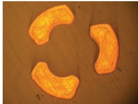
Au/Ni BARRIER (UNIFORM PLATING THICKNESS)
