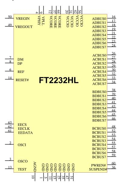
Figure 3.1 FT2232H Schematic Symbol
