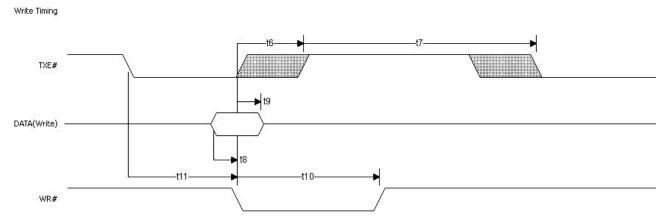
Figure 4.6 FT245 asynchronous FIFO Interface WRITE Signal Waveforms
