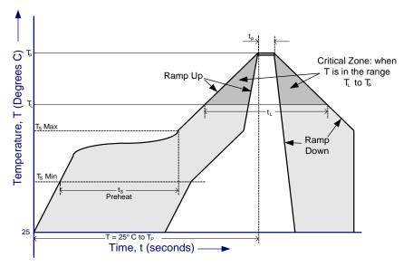
Figure 8.4 FT2232H Solder Reflow Profile
