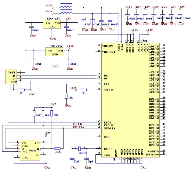
Figure 6.2 Bus Powered Configuration Example 2
