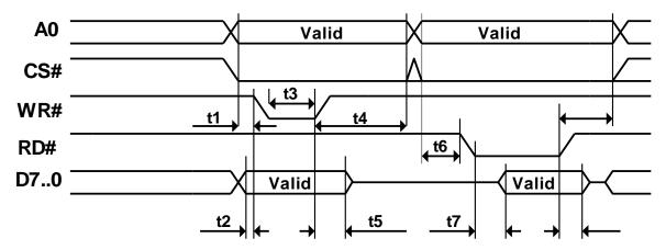
Figure 4.17 CPU-Style FIFO Interface Operation Signal Waveforms.
