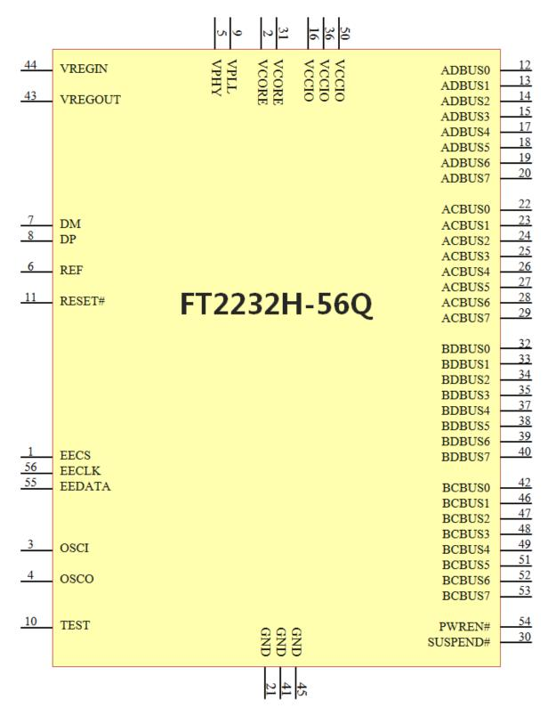
Figure 3.2 FT2232H-56Q Schematic Symbol
