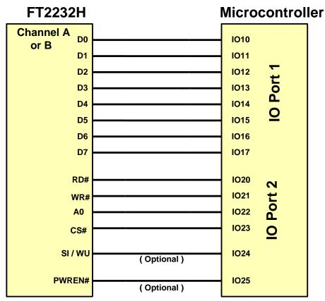
Figure 4.18 CPU-Style FIFO Interface Example
