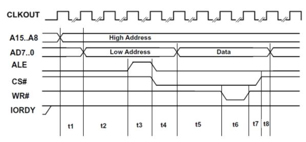
Figure 4.10 MCU Host Bus Emulation Mode Signal Waveforms - write cycle
