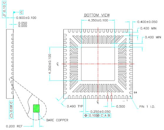
Figure 8.1 64 pin QFN Package Details
