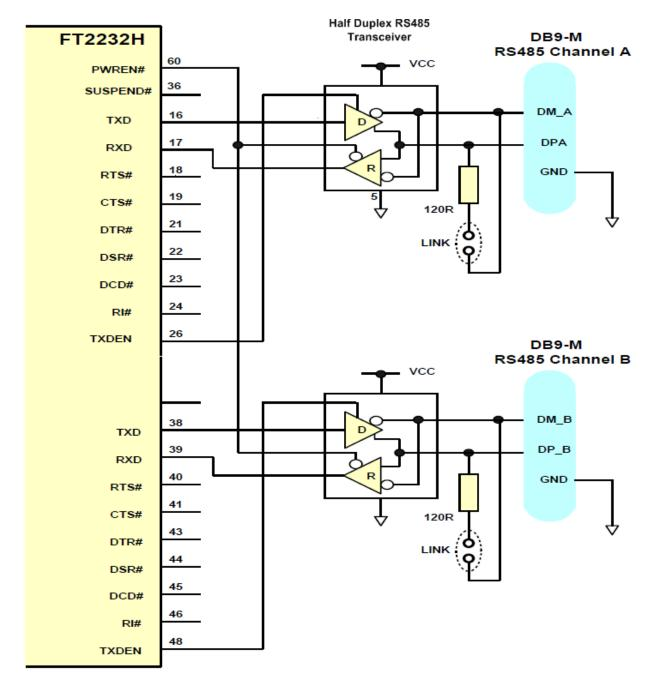
Figure 4.3 Dual RS485 Configuration
