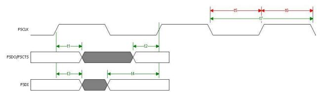
Figure 4.13 Fast Opto-Isolated Serial Interface Signal Waveforms
