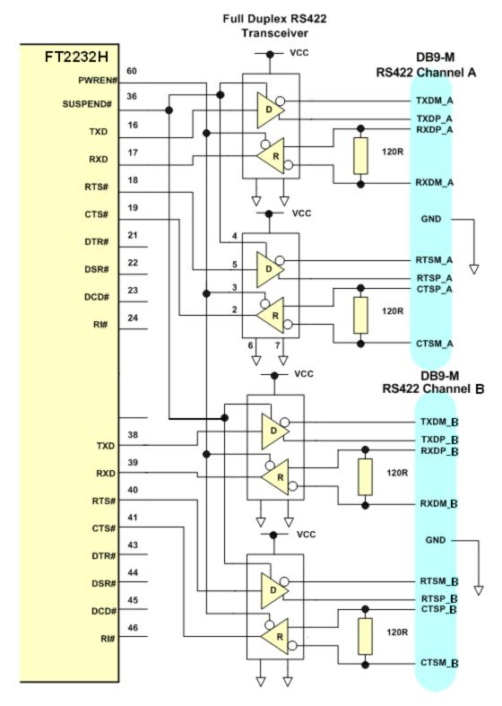
Figure 4.2 Dual RS422 Configuration
