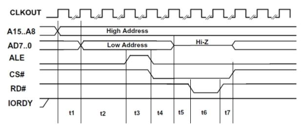
Figure 4.11 MCU Host Bus Emulation Mode Signal Waveforms - read cycle
