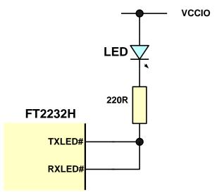
Figure 4.22 Single LED UART Configuration
