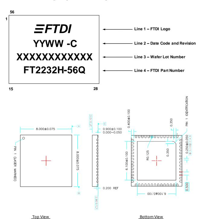
Figure 8.3 56-pin VQFN Package Details for FT2232H-56Q
