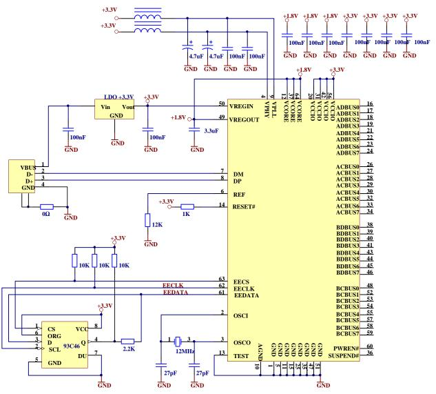
Figure 6.1 Bus Powered Configuration Example 1
