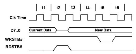
Figure 4.19 Synchronous Bit-Bang Mode Timing Interface Example
