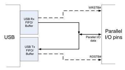
Figure 4.20 Bit-bang Mode Dataflow Illustration Diagram.
