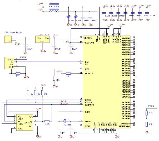
Figure 6.3 Self Powered Configuration Example 1
