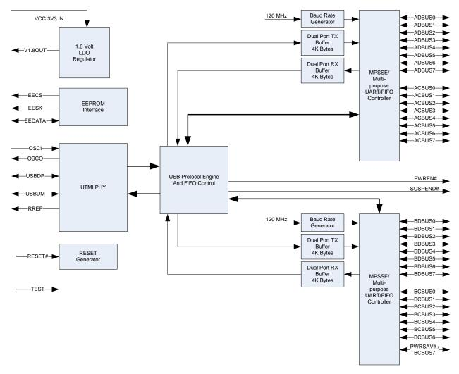
Figure 2.1 FT2232H Block Diagram
