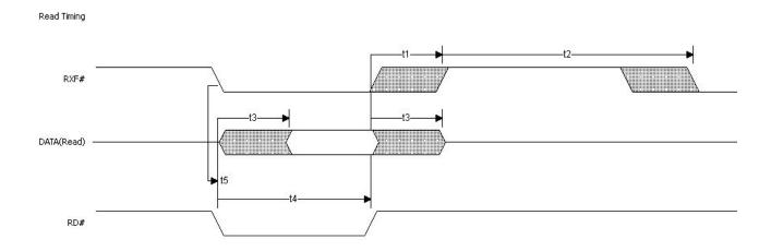
Figure 4.5 FT245 asynchronous FIFO Interface READ Signal Waveforms
