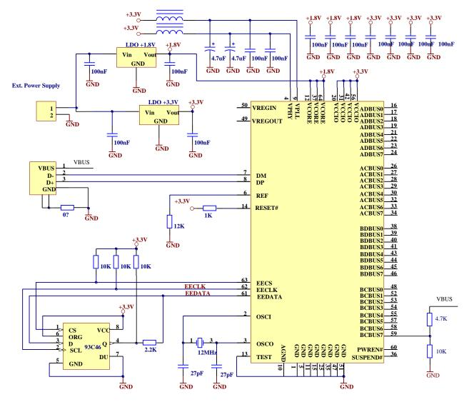
Figure 6.4 Self Powered Configuration Example 2
