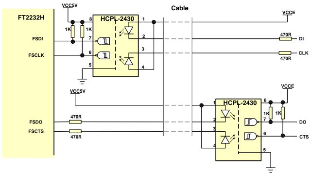
Figure 4.16 Fast Opto-Isolated Serial Interface Example
