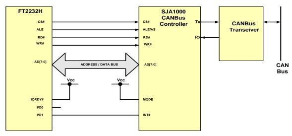
Figure 4.12 MCU Host Emulation Example using a CANBus Controller
