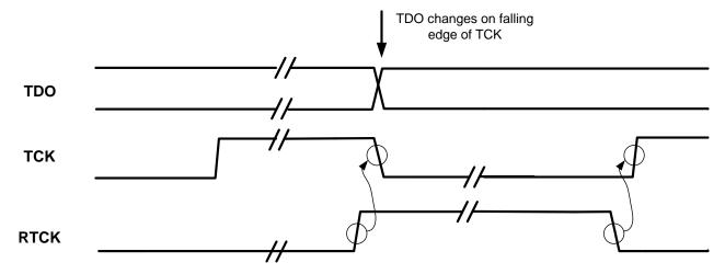
Figure 4.9: Adaptive Clocking waveform.
