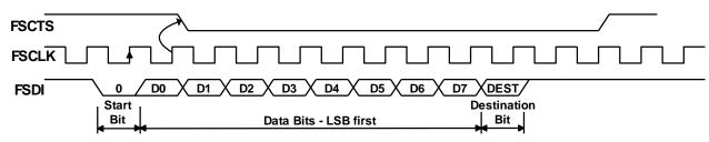
Figure 4.15 Fast Opto-Isolated Serial Interface Input Data
