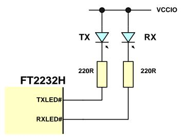
Figure 4.21 Dual LED UART Configuration
