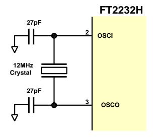
Figure 6.5 Recommended FT2232H Crystal Oscillator Configuration.
