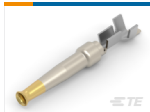
TE Part #745253-3 D-Sub Conn Contacts: Socket, Phosphor Bronze, Signal, Size 20
