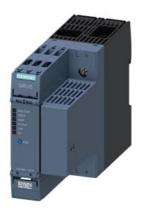
DC load monitoring relay for PROFINET, max. 1x63 A DC, max. 60 V Width: 45.0 mm Monitoring for violation of upper and lower limit of current, voltage and power; energy consumption counter, energy recovery counter, switching cycle counter, operating hours counter warning and alarm thresholds auto-reset or manual reset ON delay 0-999.0 sec, OFF delay 0-999.0 sec, automatic reclosing delay 0-999.0 sec Supply voltage: 24 VDC 1 change-over contact, screw terminal
