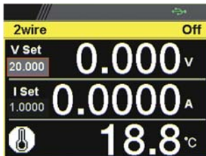
White: Temperature Control on with GTL-205A Connected
