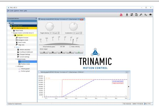
Figure 4: Driving the motor in velocity mode (TMCL-IDE provides similar view for TMC2590-EVAL)
