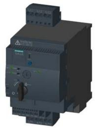
SIRIUS, COMPACT STARTER, REVERSING STARTER 400 V, 110 ... 240 V AC/DC, 50 ... 60 HZ, 8 ... 32 A, IP20, MAIN CIRCUIT CONNECTION: SPRING-LOADED TERMINAL, AUXILIARY CIRCUIT CONNECTION: SPRING-LOADED TERMINAL
