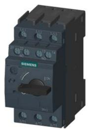
CIRCUIT-BREAKER SZ S00, FOR TRANSFORMER PROT. A-RELEASE 1.8...2.5A, N-RELEASE 52A SCREW CONNECTION, STANDARD SW. CAPACITY W. TRANSVERSE AUX. SWITCH 1NO+1NC
