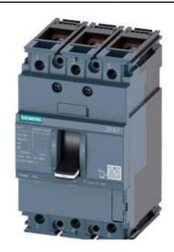
CIRCUIT BREAKER 3VA1 IEC FRAME 160 BREAKING CAPACITY CLASS N ICU=25KA @ 415 V 3-POLE, LINE PROTECTION TM210, FTFM, IN=125A OVERLOAD PROTECTION IR=125A FIXED SHORT CIRCUIT PROTECTION II=10 X IN BUSBAR CONNECTION
