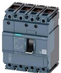
CIRCUIT BREAKER 3VA1 IEC FRAME 160 BREAKING CAPACITY CLASS H ICU=70KA @ 415 V 4-POLE, LINE PROTECTION TM210, FTFM, IN=50A OVERLOAD PROTECTION IR=50A FIXED SHORT CIRCUIT PROTECTION II=10 X IN NEUTRAL UNPROTECTED BUSBAR CONNECTION
