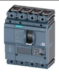
CIRCUIT BREAKER 3VA2 IEC FRAME 160 BREAKING CAPACITY CLASS M ICU=55KA @ 415 V 4POLE, LINE PROTECTION ETU860, LSIG, IN=100A OVERLOAD PROTECTION IR=40A ...100A SHORT CIRCUIT PROTECTION ISD=0,6..10X IN, II=1,5..12X IN NEUTRAL PROTECTION ADJUSTABLE (OFF, UPTO 160%) GROUNDFAULT, SWITCHABLE IG=0,2... 1 X IN, TG=0,050,8MS CABLE CONNECTION
