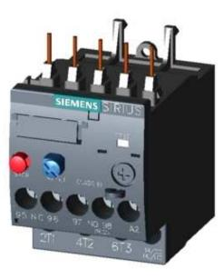
OVERLOAD RELAY 9.0...12.5 A FOR MOTOR PROTECTION BGR S00, CLASS 10 FOR MOUNTING ONTO CONTACTORS MAIN CIRCUIT: SCREW TERMINAL AUXILARY CIRCUIT:SCREW TERMINAL MANUAL-AUTOMATIC-RESET
