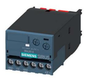
SOLID-STATE TIME-DELAY AUXILIARY SWITCH, OFF-DELAY WITH AUXILIARY VOLTAGE RELAY 1 CO CONTACT 24...240V AC/DC TIME RANGE 0.05...100S FOR SNAPPING ONTO THE FRONT; FOR 3RT2 S00-S2 CONTACTORS SCREW TERMINALS INTEGRATED VARISTOR FOR DAMPING CONTACTOR COILS
