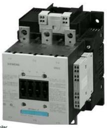
CONTACTOR, 55 KW / 400 V / AC-3 AC(40...60HZ)/DC-BETAETIGUNG UC 500-550V AUXILIARY CONTACTS 2NO+2NC 3-POLE, SIZE S6 BAR CONNECTIONS CONVENTIONAL OPERATING MECHAN. CAGE CLAMP CONNECTION
