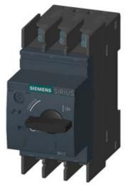
CIRCUIT-BREAKER SZ S00, FOR MOTOR PROTECTION, CLASS 10, A-REL. 0.28...0.4A, N-RELEASE5.2A RING CABLE LUG CONNECTION STANDARD SW. CAPACITY
