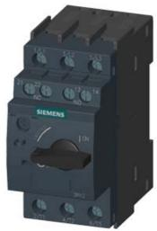
CIRCUIT-BREAKER SZ S00, FOR TRANSFORMER PROT. A-RELEASE 10...16A, N-RELEASE 286A, SCREW CONNECTION, STANDARD SW. CAPACITY W. TRANSVERSE AUX. SWITCH 1NO+1NC
