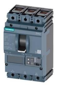
CIRCUIT BREAKER 3VA2 IEC FRAME 100 BREAKING CAPACITY CLASS C ICU=110KA @ 415 V 3POLE, LINE PROTECTION ETU860, LSIG, IN=40A OVERLOAD PROTECTION IR=16A ...40A SHORT CIRCUIT PROTECTION ISD=0,6..10X IN, II=1,5..12X IN NEUTRAL PROTECTION OPTIONAL WITH EXT. CT,UPTO 160% GROUNDFAULT, SWITCHABLE IG=0,2... 1 X IN, TG=0,050,8MS CABLE CONNECTION
