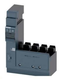
RCD- MODULE RCD510 BASIC RCD TYPE A SIDE MOUNTED ADJUSTABLE 0,03...5A AT 50/60HZ ADJUSTABLE TV 0...1000MSEC 4- POLE IN=160A UE=127-480V ACCESSORY FOR: 3VA1 WITH CABLE LUG
