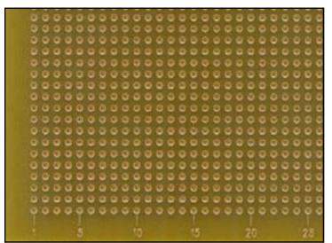
**Prototyping Board** With grid of gold plated holes.
