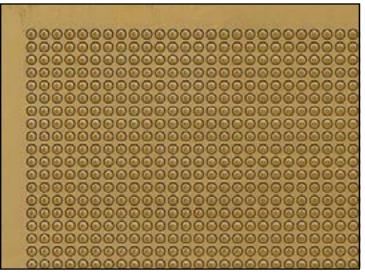
**Prototyping Board** With gold plated holes & power/ground planes. Part Numbers:
