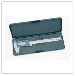
Durable stainless steel construction with sturdy padded case and locking thumb screw for precise & repeat measurement. Zero calibration switch with automatic on / off easy to read LCD screen. Metric & Imperial graduations / display with accuracy of +/- 0.02mm. Suitable for internal, external, depth and stop measurements. Maximum measure range 6" (150mm)
